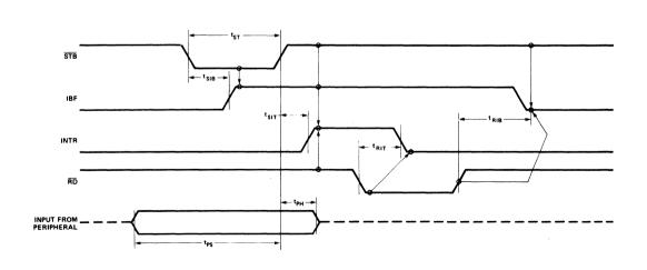
Figure 7. MODE 1 (Strobed Input)
